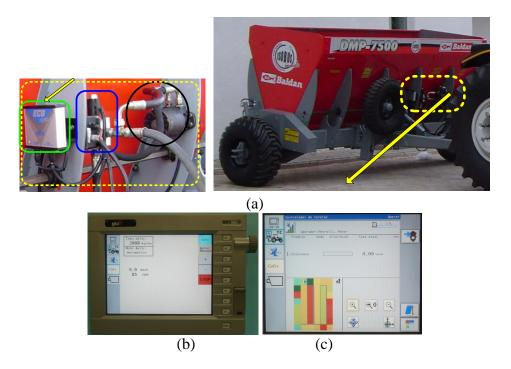
Fig. 8. (a)ISOBUS compatible limestone applicator. (b)IHM on UT to configure and control de the implement (c)VRT application according to the prescription
