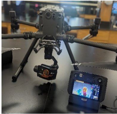
Fig. 2. DJI M300 RTK UAV equipped with Workswell WIRIS Pro thermal camera.
