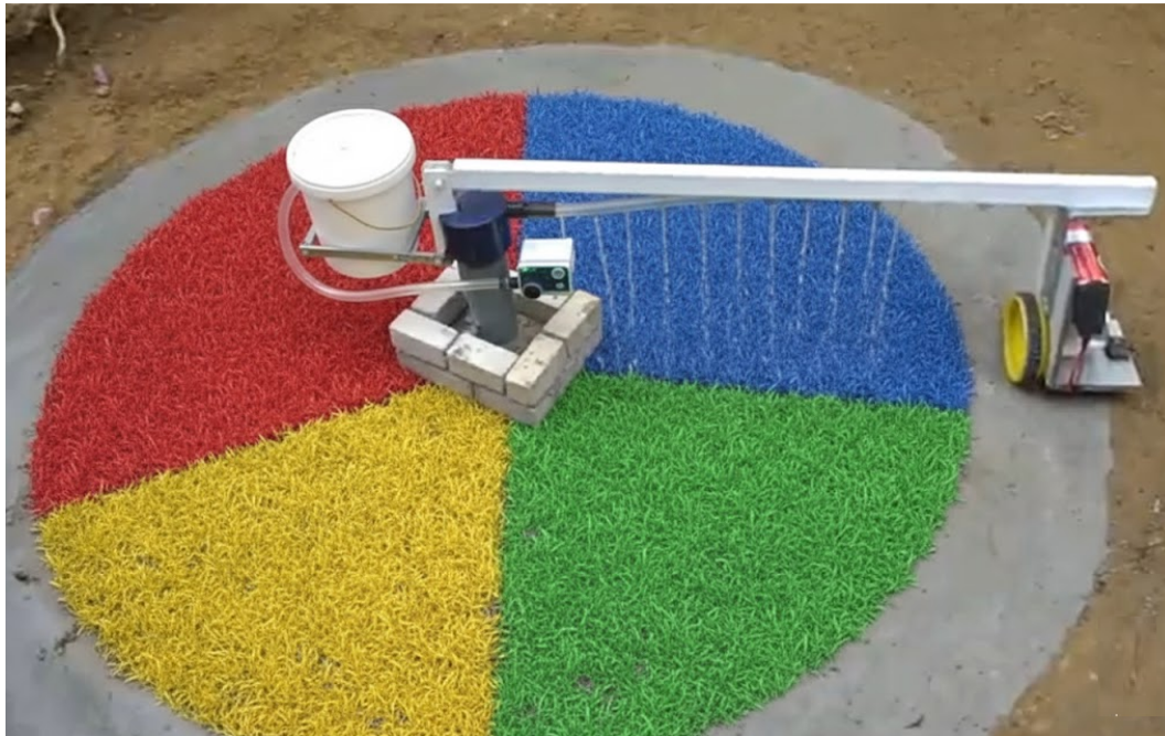
Fig 6. Implemented Scale Prototype of the Center-Pivot Irrigation System.
