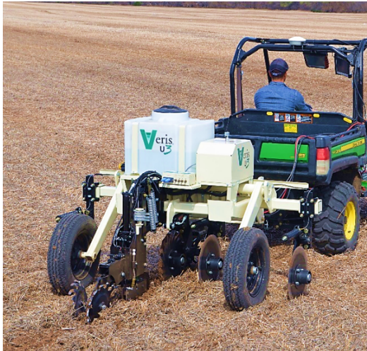
Fig. 3 Veris U3. Fig. 4 U3 pH electrodes use furrow from optical shoe
