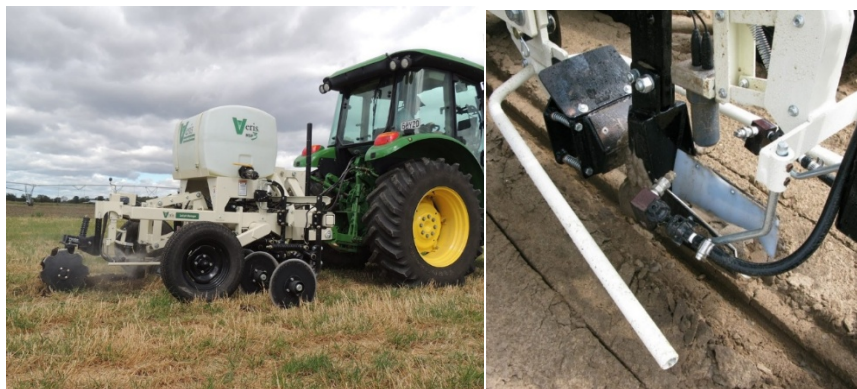
Fig. 1 MSP3 uses tractor hydraulics. Fig. 2 Soil sampling shoe collects the soil
