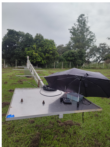
Fig. 1 Positioning of the receivers on the platform mounted at the end of the pivot
