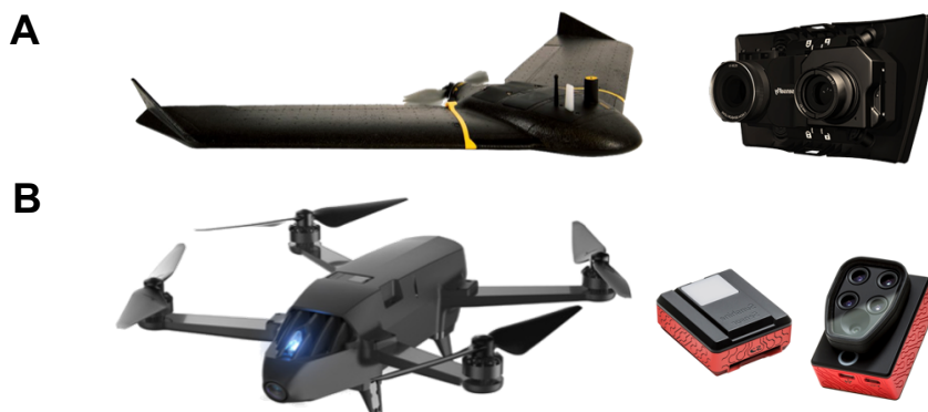
Figure 2. UAVs and sensors used in the study. A. Duet T thermal camera (left) and Ebee X fixed wing UAV (right). B. Parrot Sequoia multispectral sensor (left) and Parrot Bluegrass Fields multirotor UAV (right).
