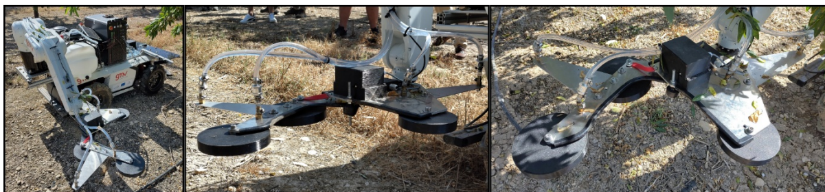
Fig. 3. Visual progression of the operation of the trunk avoidance system prototype. When contact with the tree trunk occurs, the trunk avoidance system retracts to create clearance, enabling the platform to follow its path.
