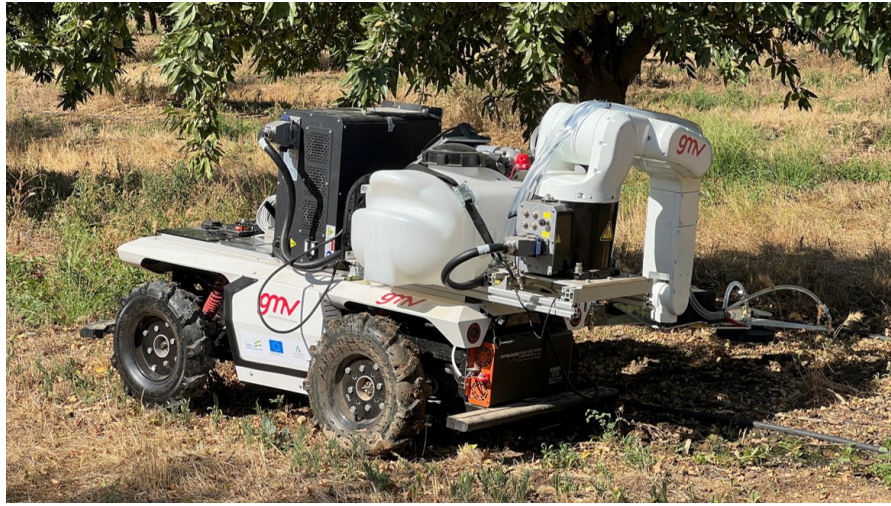
Fig. 1. Integrated robotic platform composed of: a) commercial Ackermann-steered robotic platform with IMU, RTK-GNSS and LiDAR for navigation; b) a 6-DOF robotic arm and a trunk avoidance mechanical device for reaching the intra-row space; and c) a precision spraying subsystem composed of a 20 L tank, spray nozzles, and an RGB-D camera for weed detection.
