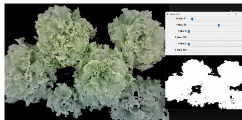
Fig. 2 Auxiliary GUI for choosing HSV inRange segmentation parameters (segmented canopy, slider controls, binary mask preview; workflow from thesis Fig. 4.9; Cheng et al., 2001)
