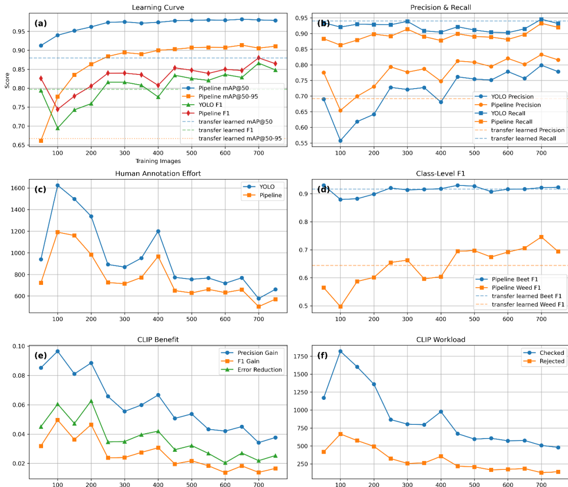
Fig. 3 Pipeline performance across 15 sequential training cycles (50–750 images). (a) Learning curves with transfer-learned fully supervised baseline. (b) Precision and recall trajectories with baseline precision and recall shown as dashed reference lines. (c) Human annotation effort measured as the number of required corrections per cycle (d) Class-level F1 scores per class with transfer-learned fully supervised baseline. (e) Per-cycle benefit of CLIP verification,
