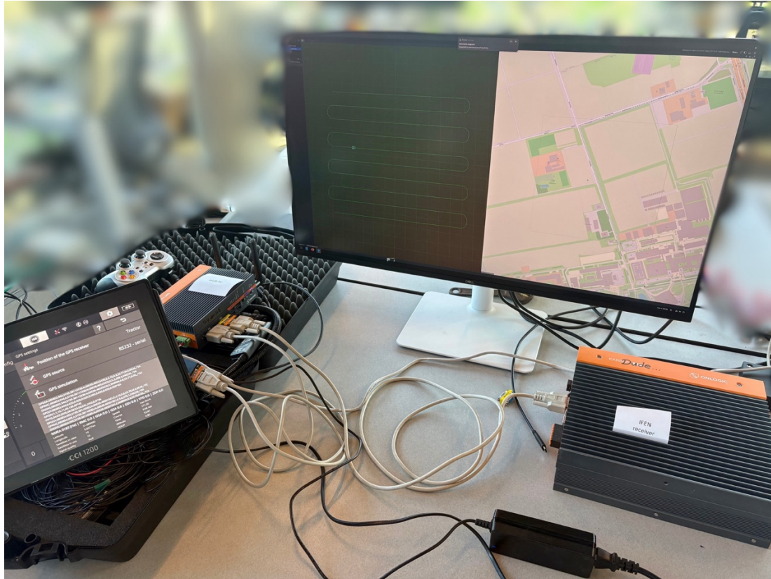
Figure 2: Test set-up. With CCI1200 terminal on the left. The WUR PC behind the CCI1200, the EPEC EC44 lays behind the CCI1200. The screen is connected to the WUR PC, the GNSS simulator on the right of the image
