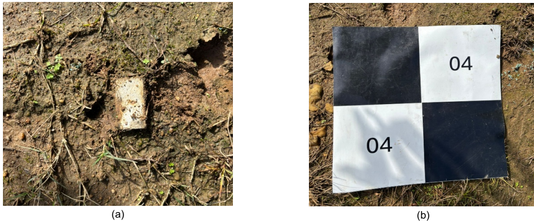
Fig 2. In (a) Identification of ground control points on the field and (b) checkerboard
