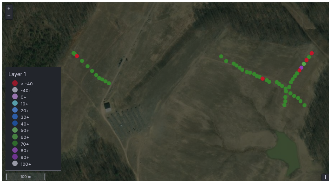
Figure 1 Placement of sensors across two growing areas: growing area 1 (left) and growing area 2 (right). Circles represent individual sensors
