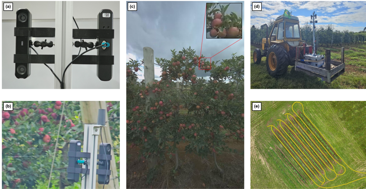
Fig 1. Data acquisition setting as seen in Santos et al. (2025): (a) stereo cameras with integrated IMU, (b) cameras oriented to the apples trees, (c) frame example, the left camera from a stereo pair, (d) the system mounted in a tractor, (e) the path registered by the GNSS system after PPK correction.
