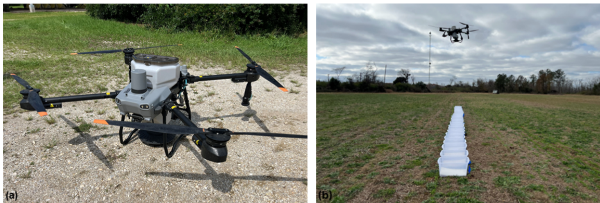
Figure 1. (a) DJI Agras T25 UAV with the dry spreading system and (b) collection pans placed within the application area and perpendicular to the UAV pass for assessing the distribution uniformity of cereal rye across the swath.
