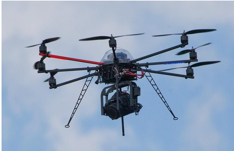
Fig 3. A RGB camera mounted on the robotic platform MikroKopter Okto XL.
