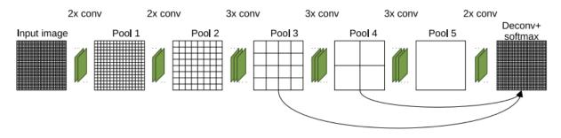
Fig 3. Overall overview of the utilized FCN model (Skovsen et al. 2017)
