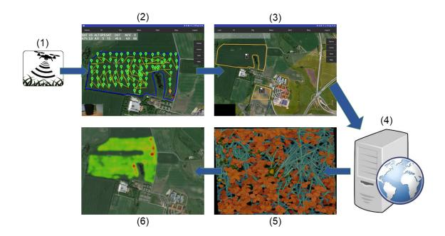
Fig 10. Dataflow of utilizing the presented model together with a commercially available UAV. The flight plan and context are controlled by an Android application and the analysis is done via cloud computing. The result is a grass-clover ratio map, which can be utilized for management of fertilization
