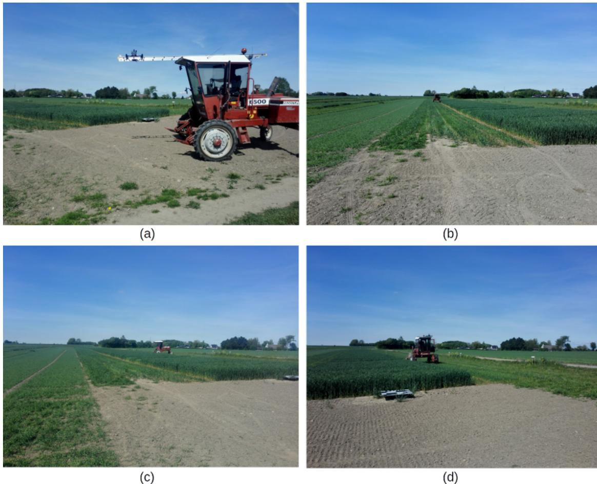
**Fig. 4** Images series documenting the recording procedure of the LiDAR data in the experimental field. (a) The starting position of the vehicle. (b/d) The recording is performed along both sides of the experimental field. (c) The vehicle drives over each fourth crop parcel.
