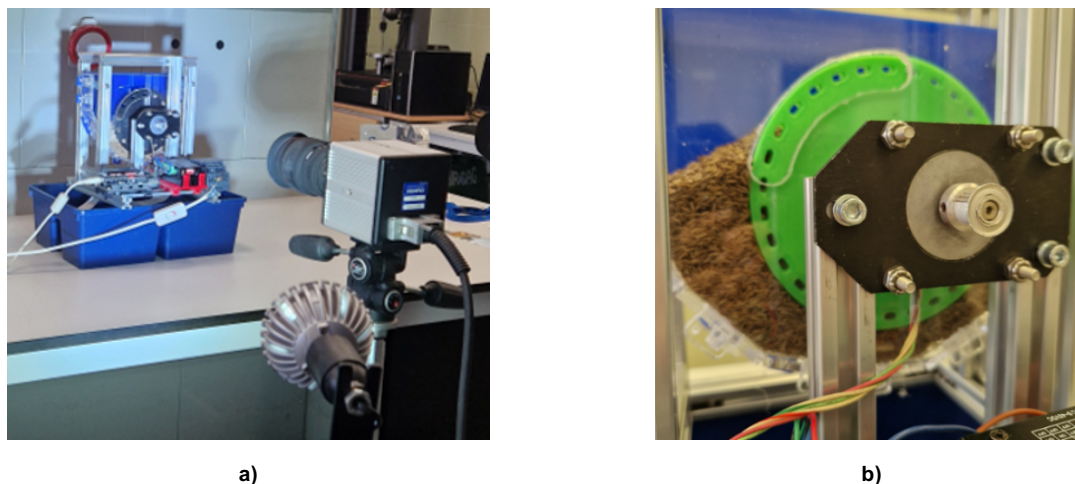
Fig 2. Experimental set up: a) general view of devices; b) seed metering unit with cumin seeds
