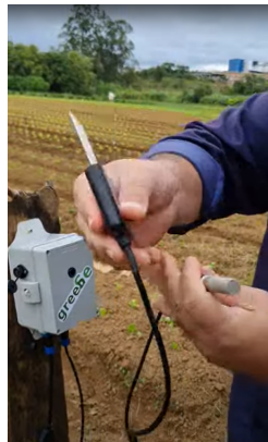
Fig. 1 RS485/Modbus RTU industrial sensors integrated in the SAGA node: 3-in-1 soil probe (temperature, moisture, EC) and SHT30 air probe (TRL-5 bench configuration)
