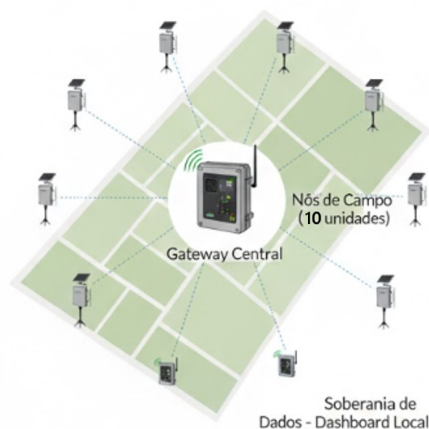
Fig. 1 Proposed architecture (not yet field-integrated): SAGA nodes, Raspberry Pi gateway, local MQTT/HTTP REST, and private IP / LoRa 915 MHz subnet (TRL-6 planned).
