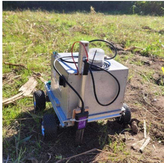
Fig. 1 Multifunctional robotic prototype developed for soil moisture data acquisition during field experiments
