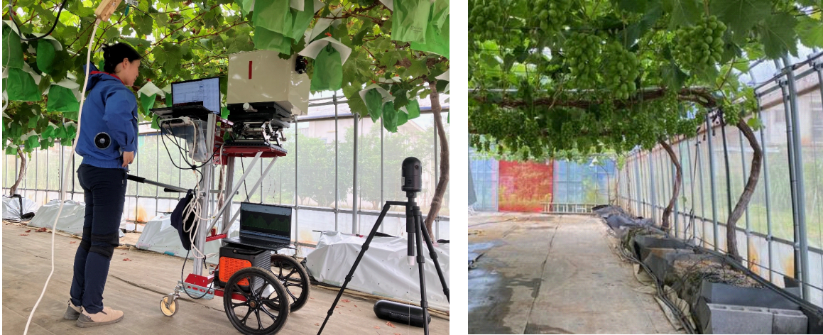
Fig 1, Developed Mid-IR spectrometer system (left), and the test field of raised-bed root-zone restriction cultivation (right).
