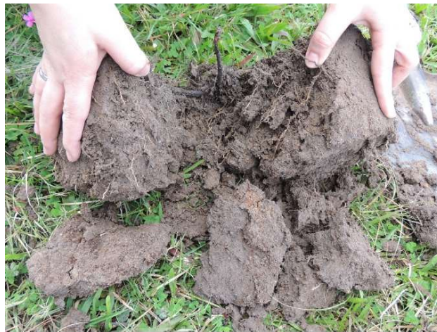
Figure 7 - A slice of soil being broken up to assess aggregation.
