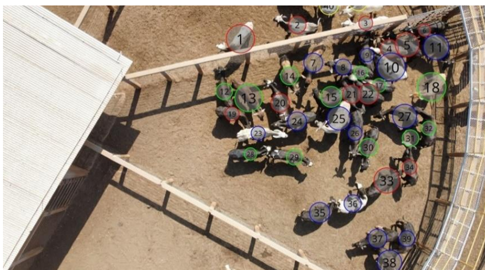
Figure 2 - Aerial visualization using RPAS, indicating cattle numbering and counts via computer vision.
